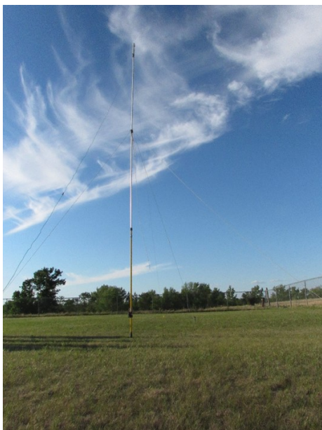
The author's 40m, end-fed, half-wave antenna, deployed in a POTA activation in North Dakota
